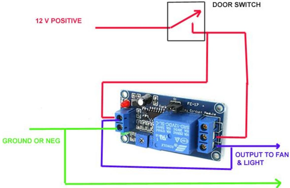
The blue line is also a feedback circuit to keep the fan & light on for the set amount of time
