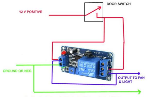
The blue line is also a feedback circuit to keep the fan & light on for the set amount of time
